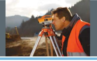
Nedo Z-Series levels are premium engineers' levels that meet the most exacting demands. The levels in this series have an especially large aperture to provide plenty of light-gathering power, a rugged, airdamped compensator and a jet-water proof metal housing conforming to protection class IP X6.
