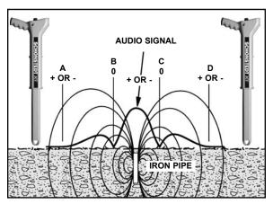
Figure 10. Signal Pattern from a Strongly Magnetized Marker
