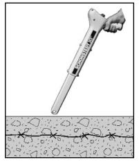
Figure 15. Tracing Barbed Wire
