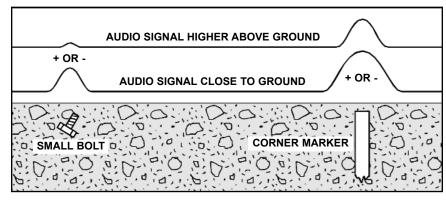
Figure 9. Decreasing gain Eliminates Unwanted Signals
