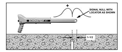
Figure 18. Placement of Locator while Searching along a Chain Link Fence
