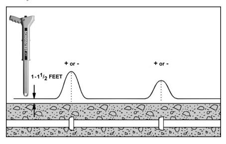
Figure 20. Signal Patterns Provided by Cast-Iron Pipes
