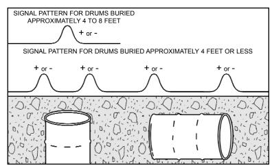
Figure 21. Signal patterns provided by steel drums
