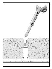
Figure 19. Locating Valve Boxes and Casings
