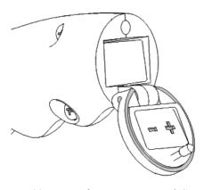
Figure 22. View of Battery Door and Compartment
