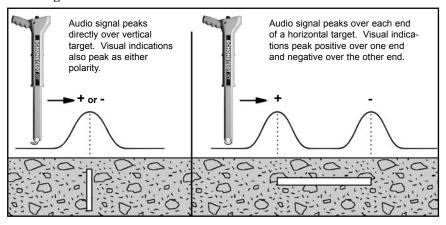
Figure 7. Signals from Vertical and Horizontal Targets
